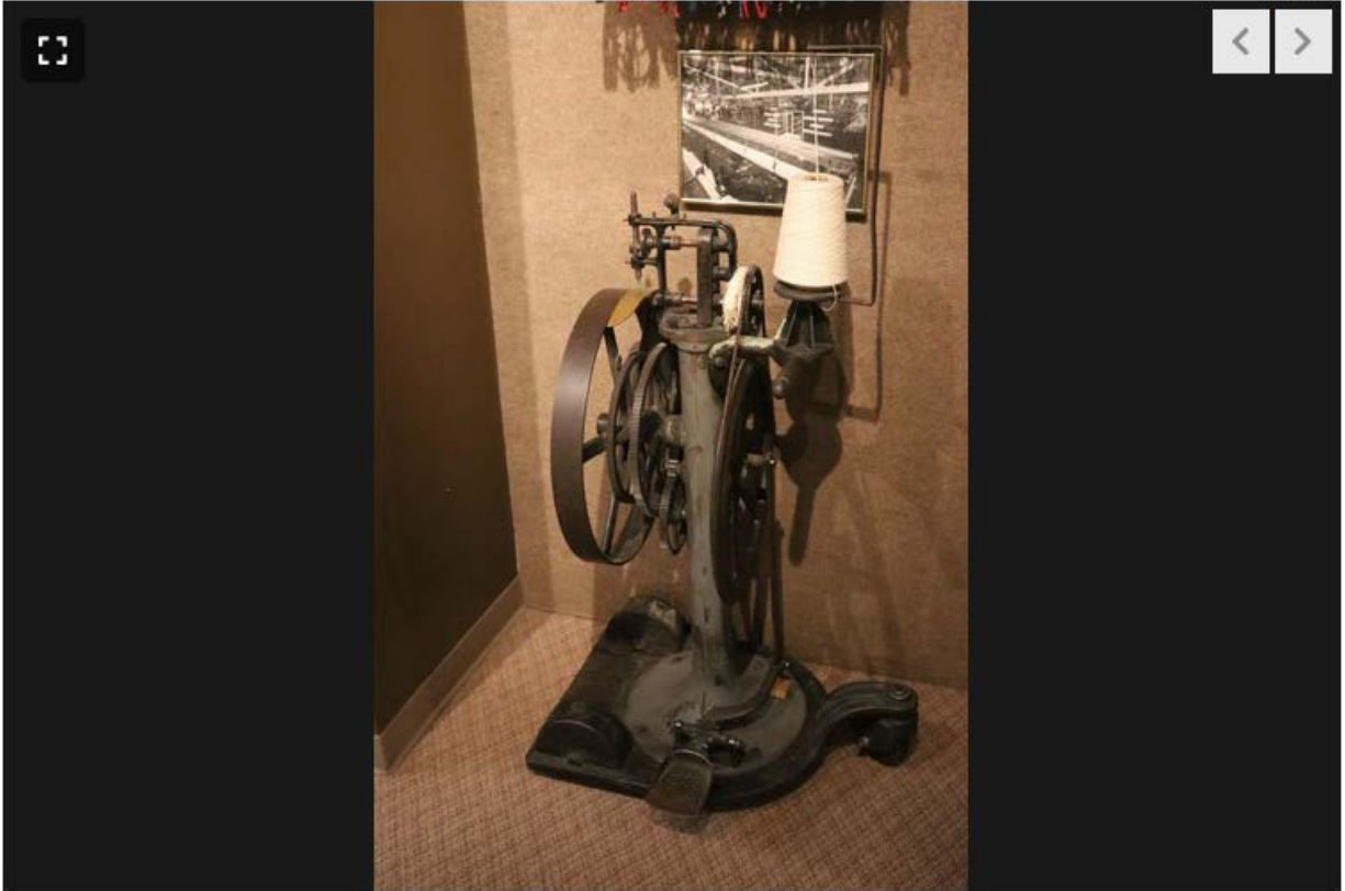
This Woolen Mills binding machine circa 1908 was used to bind the edges of blankets and powered by the floor pedal, not electricity.
