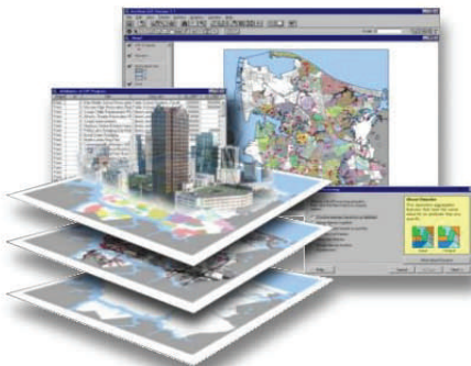
Layers of data are used to build a complete mapping system. Layers are either point, line or polygon data.
